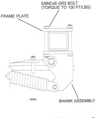
1. For ease of installation loosely assemble the frame plate to the shank assembly with the two rear bolts (Note direction of bolts).
