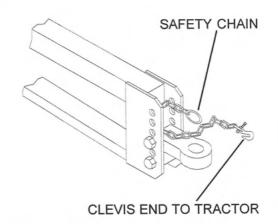
The intermediate support is to be used if there is more than 6" of unsupported chain on either side of the primary attaching point.
