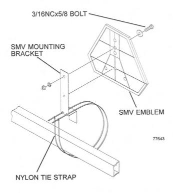
The bracket provided is designed to mount to numerous frame sizes and can be mounted in different positions to avoid interference with implement components.
