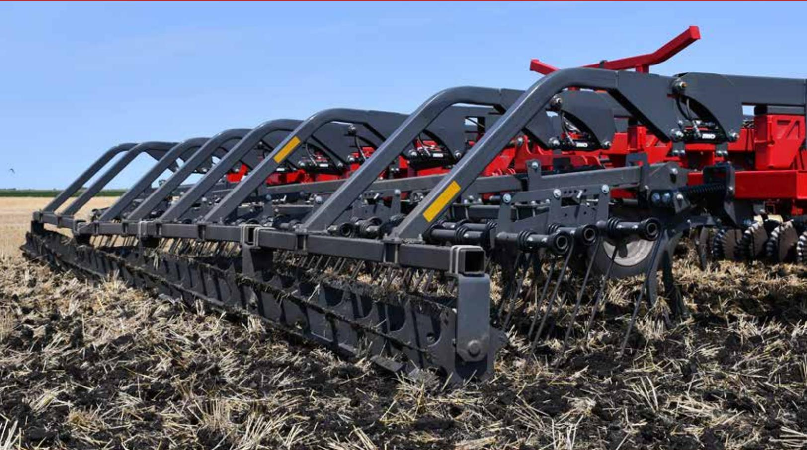
Optional leveling attachments of a three-bar harrow, four-bar harrow, or three-bar harrow with hydraulic rolling basket with adjustable down pressure, leave a smooth field finish for spring seedbed preparation.
