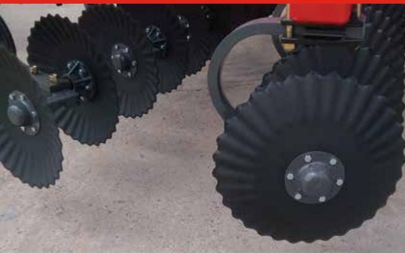
Two rows of double-mounted discs can be set for desired depth independent of the shanks. Concave razor blades are 24 inches (61 cm) in diameter and spaced 15 inches (38 cm) apart. The second rank of blades is offset from the first for effective spacing of 7½-inches (19 cm).
