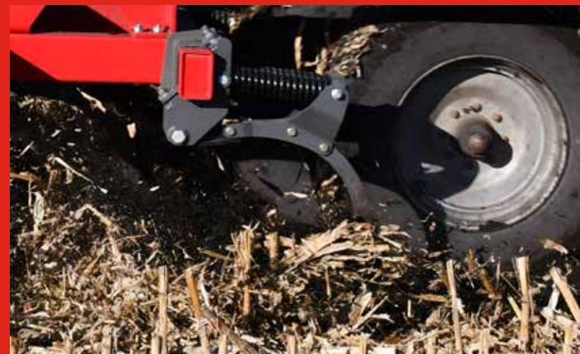
Four ranks of 1400-pound (635 kg) trips with on-edge chisel shanks give additional dragging and mixing after the discs. Sixty-inch (152 cm) spacing between shanks on each of the ranks allows for excellent trashflow through the tool. The overall 15-inch (38 cm) spacing aids in a smoother field than the typical wider shank spacing of disc rippers.
